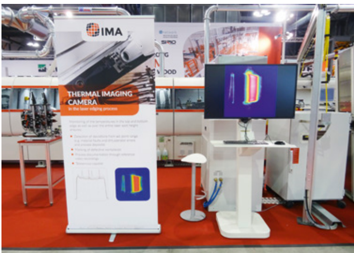
Monitoring optimal laser edging with the help of a thermal imaging camera at Ima.
