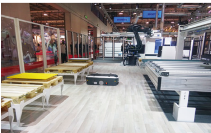
Homag demonstrated its "autonomous cell" with a driverless vehicle that provides material to a robot that then puts the goods on the machining centre and takes them off again.
